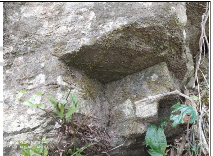
H) Rock wedge came out due to favorable joint interference (12°10'1.28"N/75°43'16.79"E)
